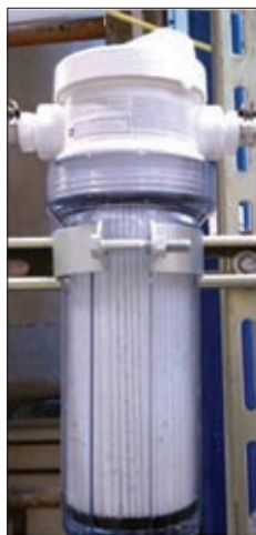
Left: Figure 1. Depiction of electropositive filtration media. Center: Figure 2. Pleated cartridge containing the Ahlstrom electropositive filter.
