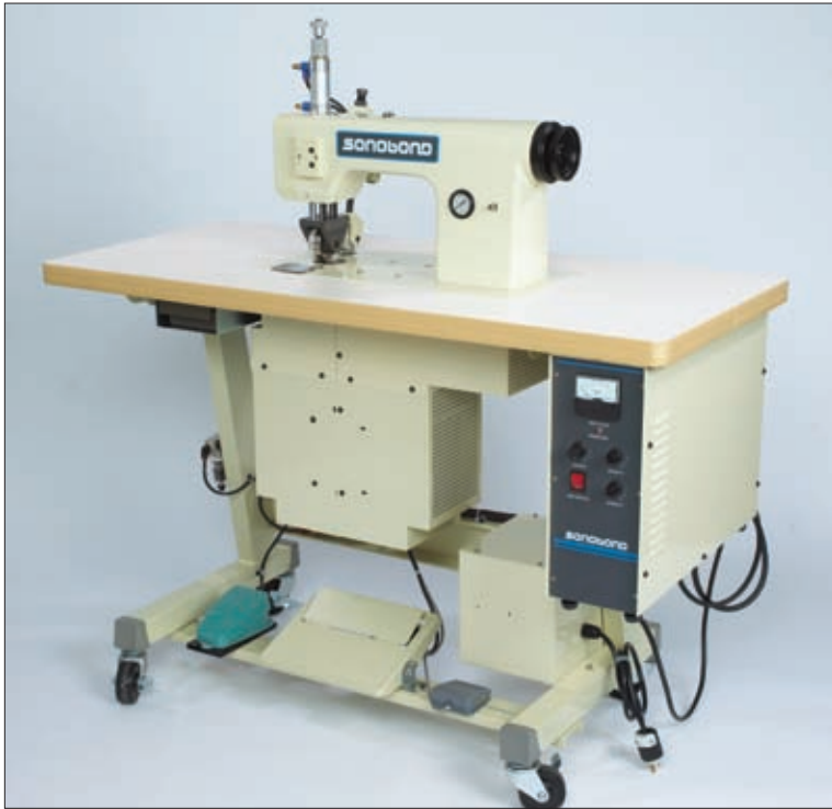
Sonobond's SeamMaster High Profile Ultrasonic Bonder is an easy-to-operate machine and is available with a special fixture for bonding pleated filters. It is used to assemble jet fuel filters, commercial air filters, oil-absorbent booms, and much more.
