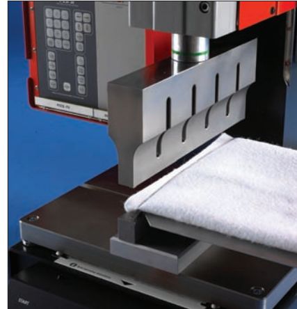
JL Filtration uses Sonobond Ultrasonics' PlungeBonder to seal the ends of filter bags.
