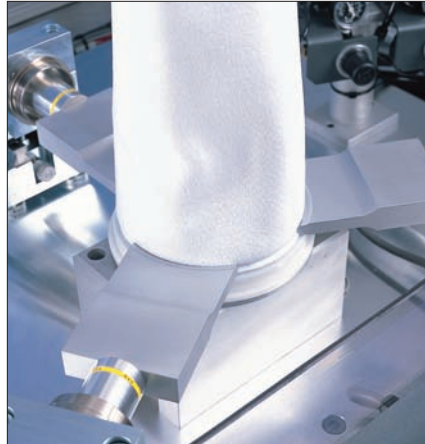
PlungeBonder welding the end of a filter bag.
