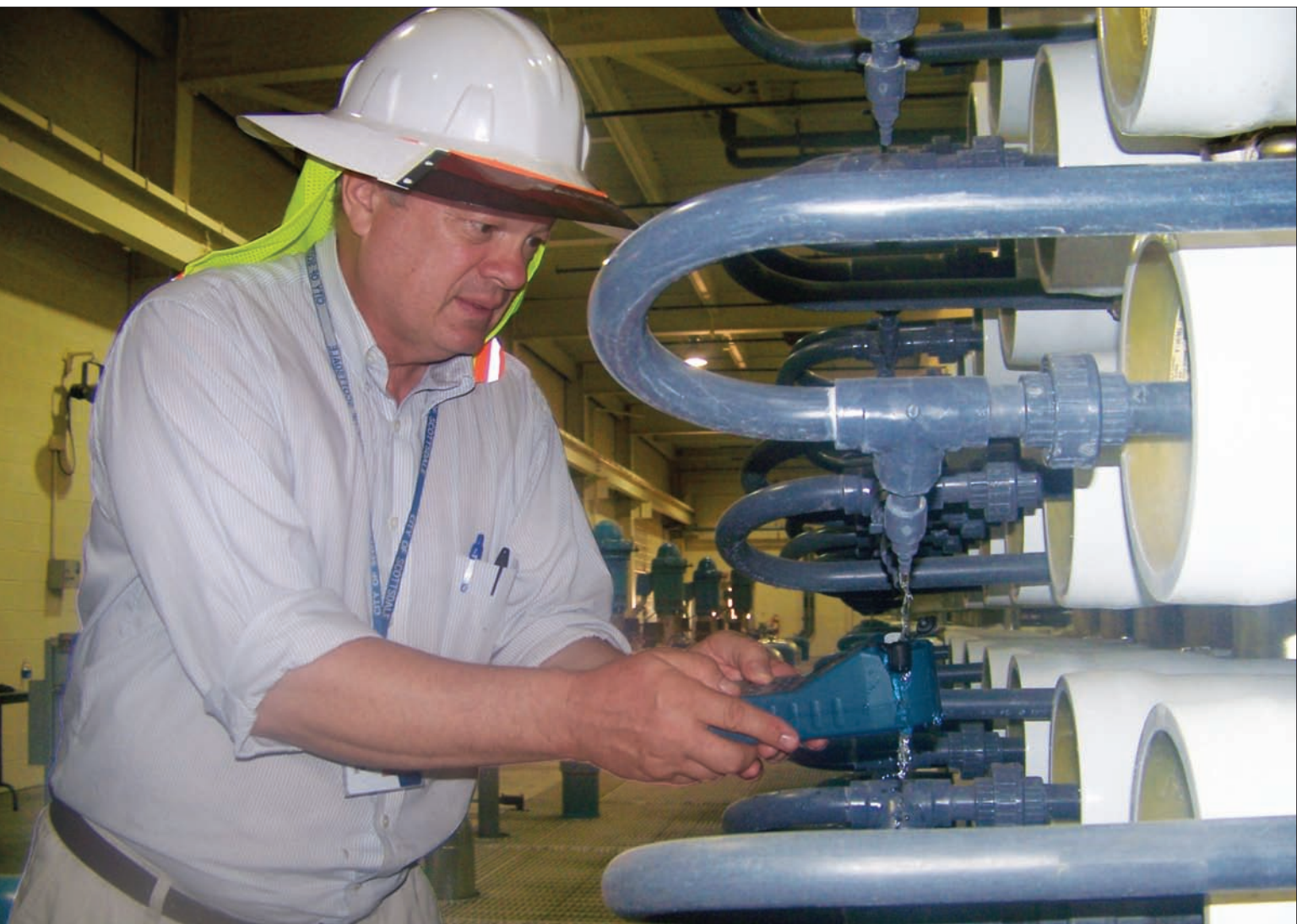
Figure 1: The New 9P Titration Kit from Myron L Company features conductometric titrations for on-the-spot analysis of hardness, alkalinity and saturation index.
