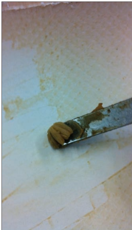
Fig. 3: R.O. membrane surface close up, removing solids from membrane surface.
