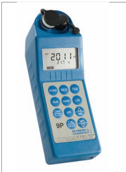
Figure 3: The Ultrameter III 9P gives a numerical digital reading that requires no interpretation, while colorimetric tests require the user to determine the endpoint by color change, which can sometimes be missed while trying to keep track of reagent additions.
