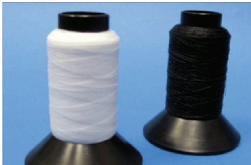
Figure 3. PTFE thread twisted from slit film monofilament – Black pigmented and White unpigmented.
