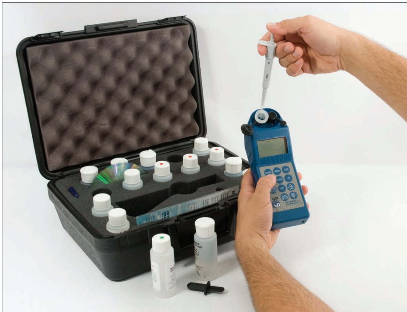
Figure 4: The 9PTK comes with everything you need to analyze Conductivity, Resistivity, TDS, pH, ORP, Free Chlorine, Temperature, Alkalinity, Hardness, and LSI in the field.
