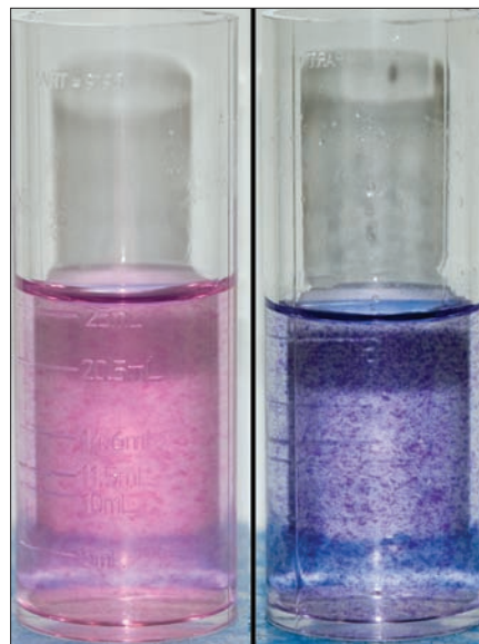
Figure 3: The Ultrameter III 9P gives a numerical digital reading that requires no interpretation, while colorimetric tests require the user to determine the endpoint by color change, which can sometimes be missed while trying to keep track of reagent additions.
