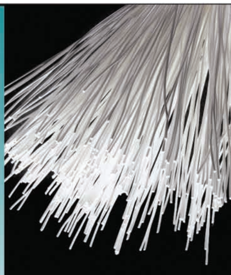
Hollow fiber membranes can be assembled into bundles
