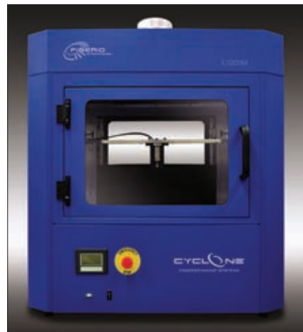
FibeRio production route is based on the 'force spinning' principle.
