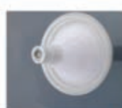
Figure 9. 8mm diameter filter holder for the Sonic Filter Tester
