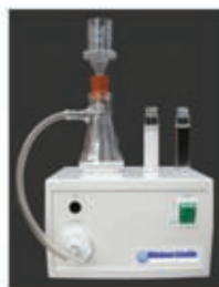
Figure 12. A simple split filter apparatus for the wet challenge test
