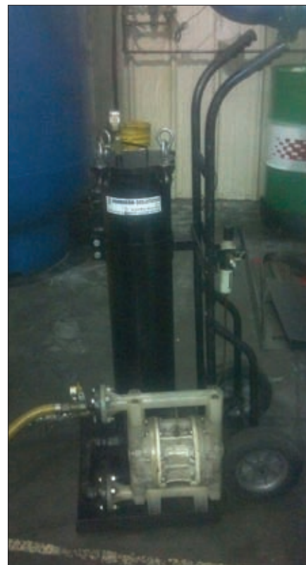
Figure 2: A typical bag filter with a pump designed to work as a sump-side cleaner on a sidearm concept.
